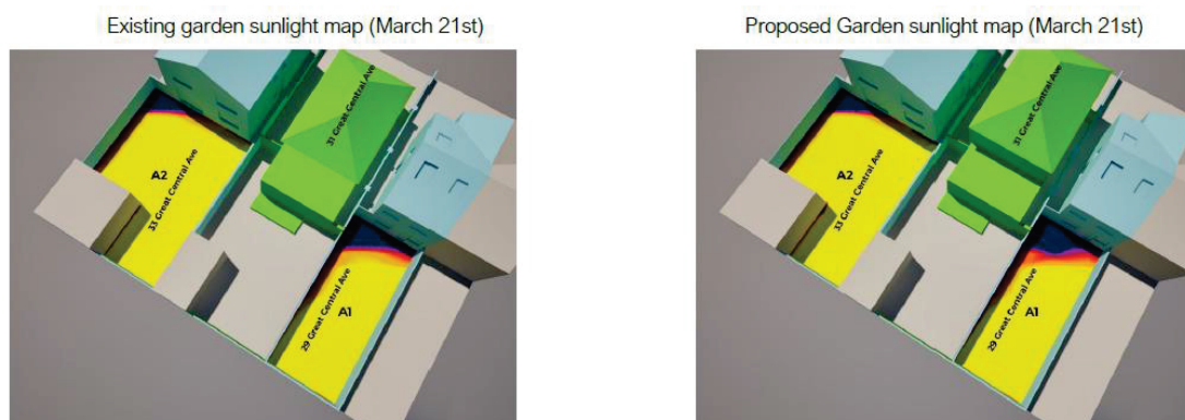
Figure 9: Sunlight map of garden sun on March 21 st as per BRE Guidance
